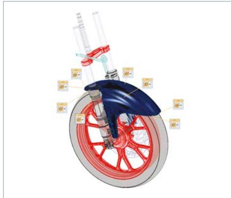
Bounded surfaces now allow guide curves for added shape control while supporting curvature continuous boundary conditions for ensuring a smooth match to adjacent faces. The user experience is elevated by taking advantage of 3D control handles and surface visualization tools, such as UV curves and curvature combs.
