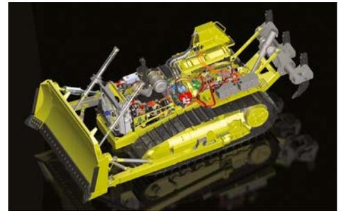
In the all-new simplify assembly environment, designers can further refine the representation of large assemblies. All ordered part modeling commands are available, as are several new tools. This functionality is especially valuable for original equipment manufacturers (OEMs) and suppliers who need to remove proprietary data from assemblies prior to sending the models to final product manufacturers.
