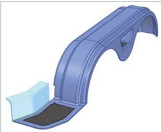
Another enhancement in stamped metal design enables contour flanges to be defined on the edges of existing contour flanges.
