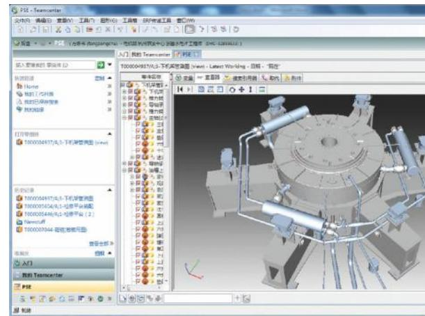
View of the lower frame assemblies of this hydropower equipment using Teamcenter.
