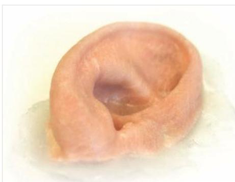
*3D printed soft tissue prosthesis created via unique process pioneered by Fripp Design and Research.*
